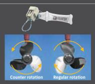
Function for selecting standard or counter rotation on one outboard with an optional connector.
