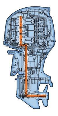
**2 STAGE GEAR RATIO REDUCTION**The Offset Driveshaft system has two stages of reduction, allowing it to turn large propellers with high efficiency,
