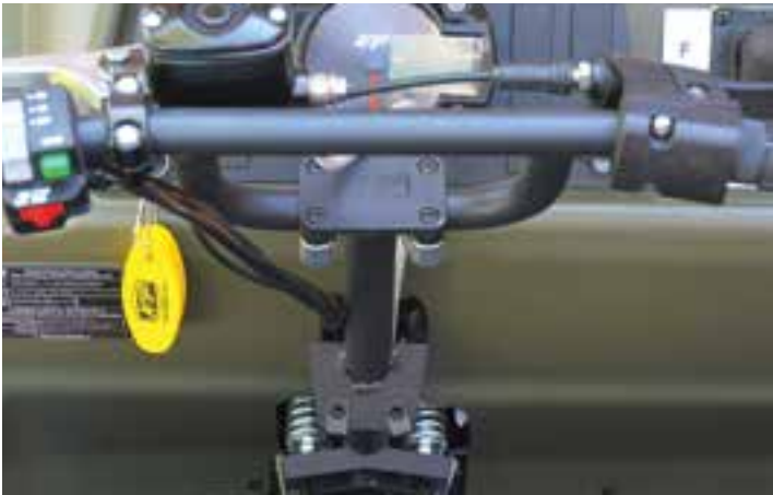
By adding a spring element between the handlebars and the brake system, we achieved a progressive dual-rate steering system.
